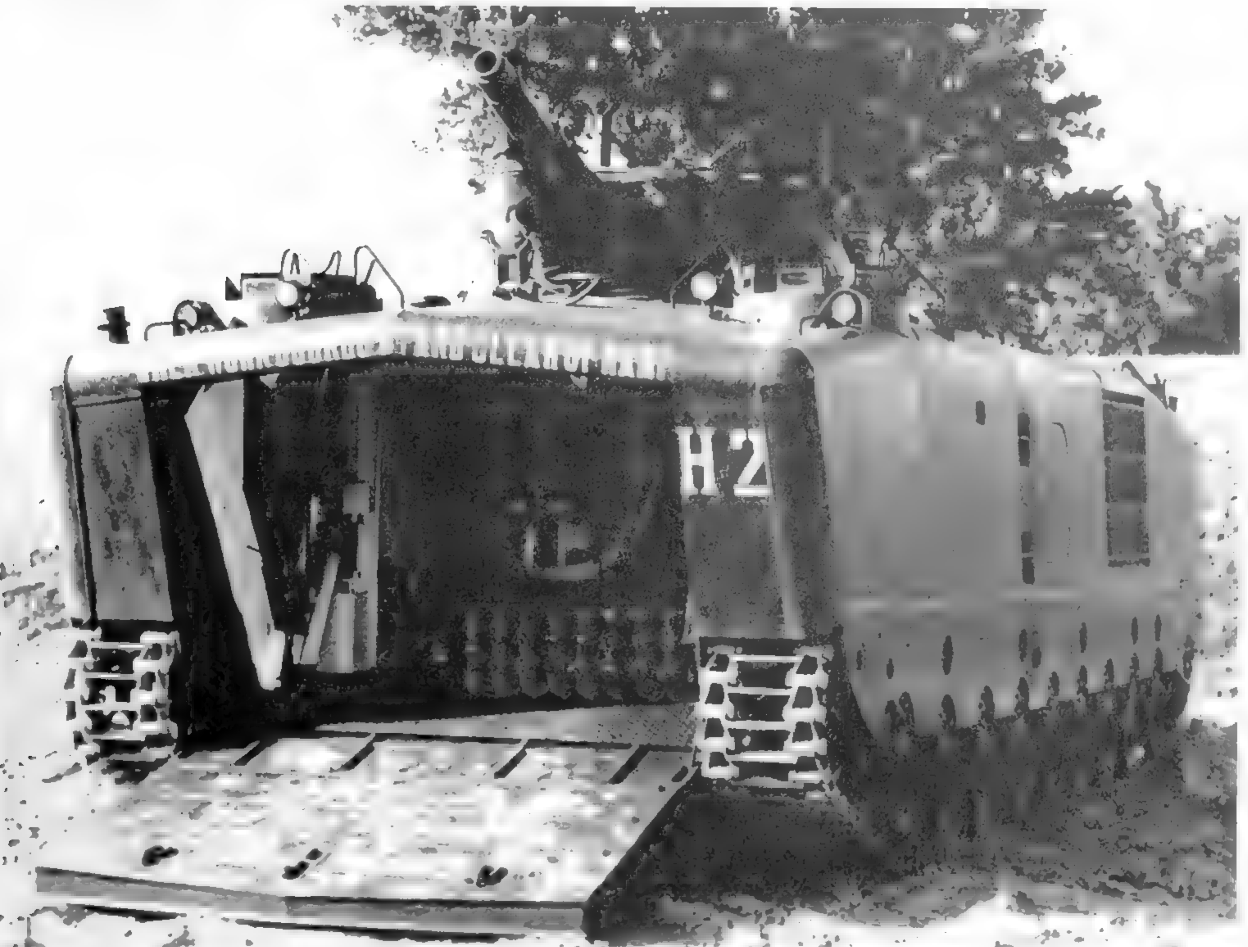
The LVTH6 was provided with stowage for 151 rounds of 105mm howitzer ammunition. One of the stowage racks is visible in this view of the vehicle front with the ramp down. When the LVTH6 was operating in water, the ammunition carried was reduced to 100 rounds. (Photo courtesy of the Patton Museum)
